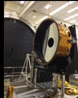
PTC control system achieved 2K accuracy with 2mK stability of 1.5-m AMTD-2 ULE® mirror
